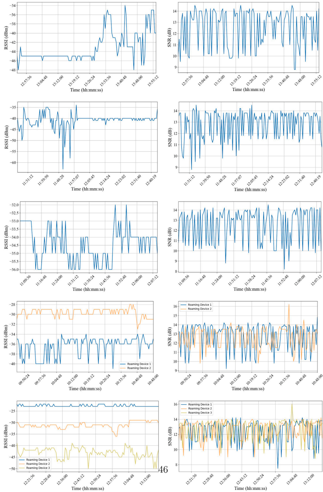
Fig. A.30. RSSI and SNR at the Chirpstack Server for the tests performed with the Golang version. From top to bottom, results for Test 1, Test 2, Test 3, Test 4, and Test 5.
