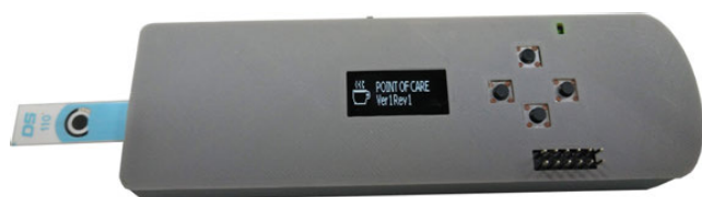
FIGURE 11. Photograph of the final assembled handheld PoC prototype.
